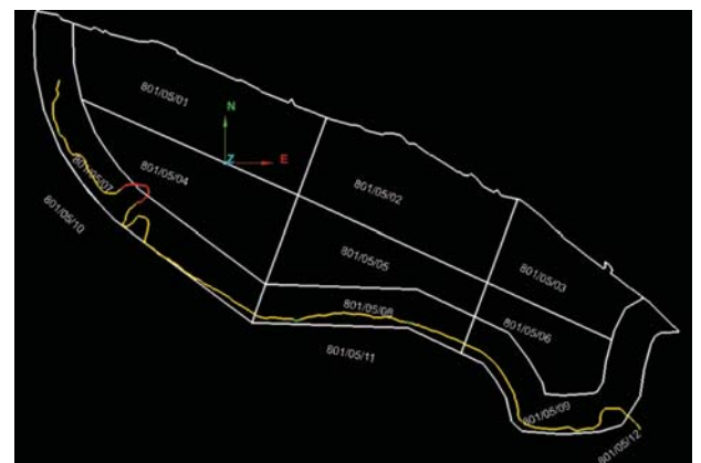
Figure 6—Example of a plan view showing actual toe line overlain on planned block design
