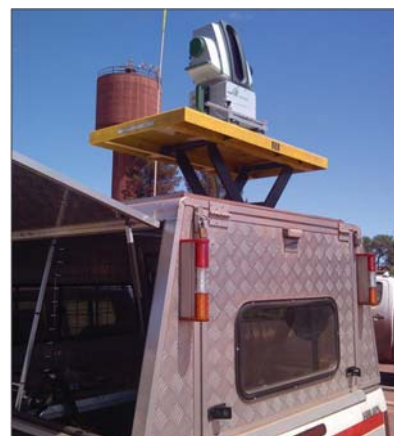
Figure 2 – Vehicle-mounted laser scanner set-up
