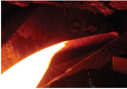
Figure 2—High-intensity water-cooled slag tap-block with solidified slag freeze lining core through which slag is tapping at 1659°C
