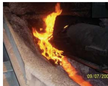
Figure 17—Excessive tap-hole clay bypass (Ndlovu et al. , 2005)
