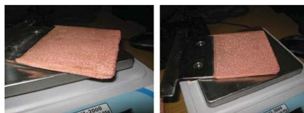
Figure 4—Bench-cell cathodes produced using TFM electrolyte at 430 A/m<sup>2</sup>
