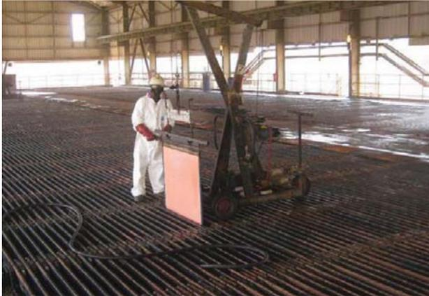
Figure 9—Single-pull cart used to correct short-circuits in tankhouse
