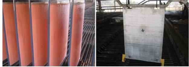
Figure 6—A-style bottom corner and blue star insulators on anodes, three-side edge strip on cathodes
