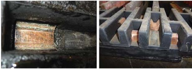
Figure 5—Old cell furniture (right), showing poor clearance between cap block and contact. On left is new cell furniture with robust contact clearance
