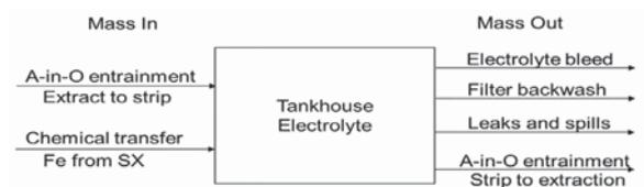
Figure 5—Mass balance streams for tankhouse electrolyte
