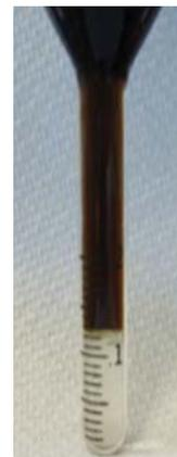
Figure 2—Centrifuge sample holder showing separated aqueous phase
