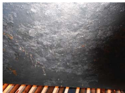
Figure 3—Hard, dense, adherent \alpha - \text{PbO}_2 (brownish colour)
