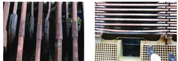
Figure 9—Uneven electrode spacing
