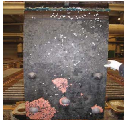
Figure 10—Copper plating on lead anode (courtesy of Nikkelwerk)
