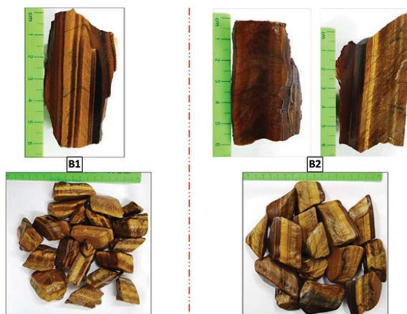
Figure 6—Polished pieces of tiger's eye (top) and tumbled products (bottom) of B-grade subtypes
