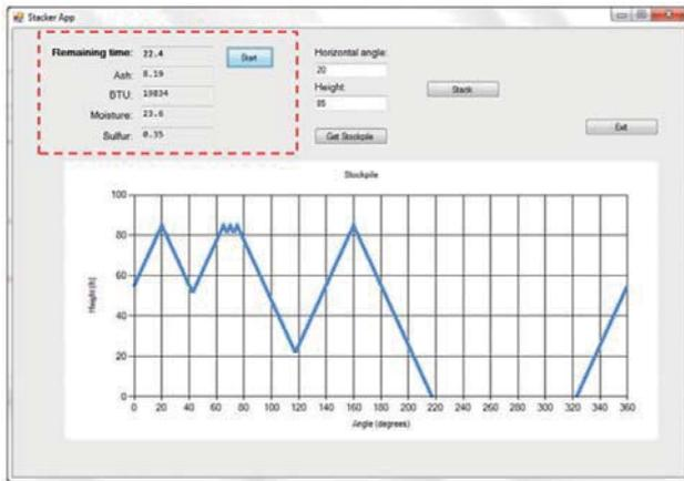
Figure 9—Remaining time and analyser real-time output window
