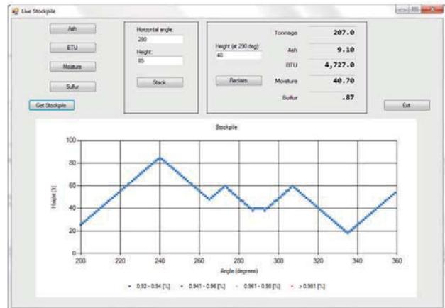
Figure 16—Stockpile's shape after reclaiming to 12 m (40 ft)
