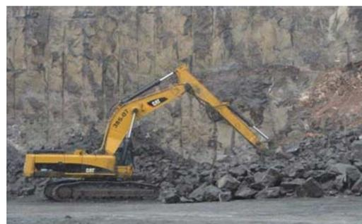
Figure 5—Scaler working on highwalls
