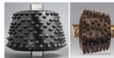
Figure 15—Rowed carbide cutter (left) and random cutter (right) (from Brooke, 2008)
