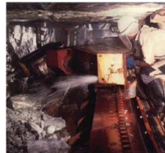
Figure 7—The impact ripper mounted on the impact mining system (from Willis, 2001)
