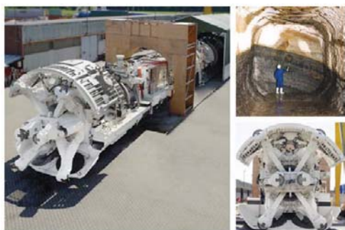
Figure 23—Wirth Mobile Tunnel Miner showing overall size, ability to cut arbitrary profiles, and arrangement of undercutting discs (AkerSolutions, 2013)
