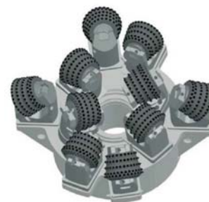
Figure 16—Arrangement of cutters on a 1.8 m raisebore head (from Brooke, 2008)
