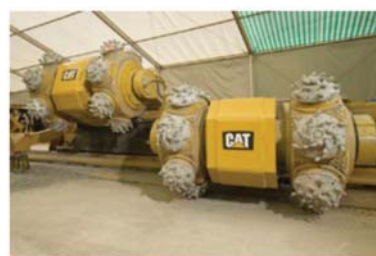
Figure 26—The Caterpillar Rock Straight System (from NarrowVeinInfo, 2015)
