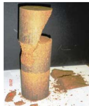
Figure 14—Compounded specimen with H/D of 3.4 after testing and after removal of loose fragments
