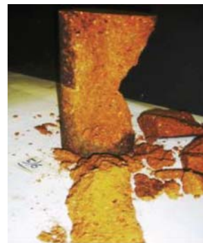
Figure 13—Compounded specimen with H/D of 2.3 after testing and after removal of loose fragments
