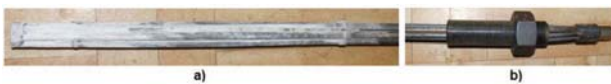
Figure 22 – Yielding bolt after the test (without damage) as a threaded cylinder liner and nut
