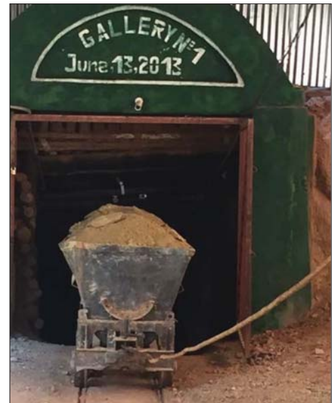
Figure 1 – 1 t hopper being hoisted out of the Incline shaft
