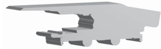
Figure 4—Simplified 3D model of the object impacting the platform – mechanized cover segment
