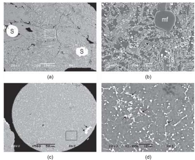
**Figure 2—**(a) Typical microstructural detail of granulated calcium ferritic slag with Cu-(Fe)-Ni-(Pd) sulphide inclusions (S). (b) Detail from Figure 2a. Ca-Fe oxides of type calcium ferrite (CF) and dicalcium ferrite (C<sub>2</sub>F). Ni-Mg-Fe-(Ca)-(Cr)-(Co) oxide of type magnesia-ferrite (mf). Sulphide inclusions (S). (c) Typical microstructural details of granulated matte. Pd, Pt-enriched Cu-Fe-Ni sulphide (arrows). (d) Detail from Figure 2c
