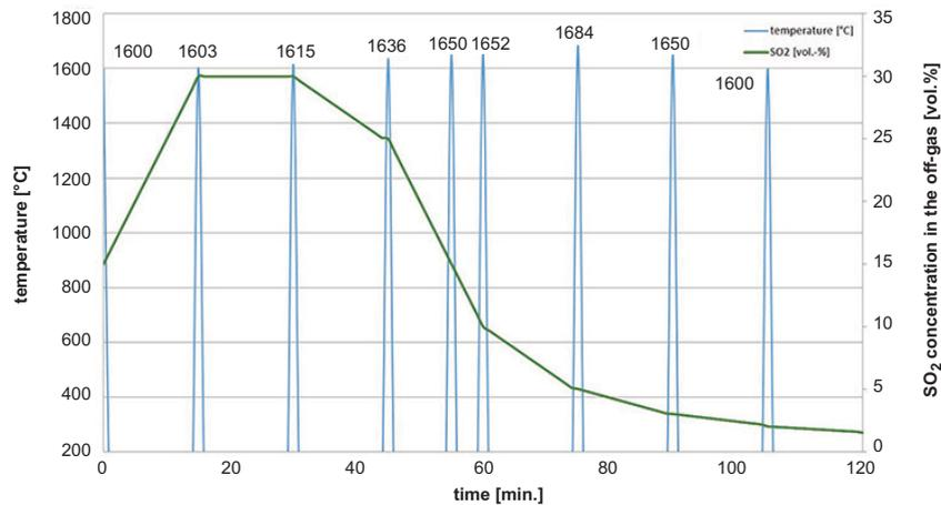
Figure 5—Example of the temperature and SO<sub>2</sub> content of the off-gas during tests 3 and 4. For process control the temperature of the liquid matte was measured (discontinuously) every 15 minutes, shown as spikes in the diagram
