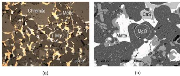
**Figure 11—Typical microstructural details of MCB6 after trials 3 and 4. Reflected-light microscopy (a) and scanning electron microscopy (b). Approximately 10 mm from the hot face. Infiltrated and corroded brick microstructure, showing corroded magnesia component (MgO), mickel matte, and idiomorphic Ca sulphate (CS)**
