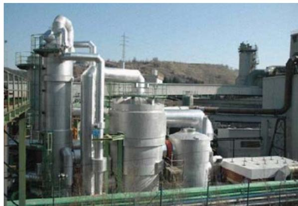
Figure 3—CORE™ installation processing gas up to 21 vol% SO<sub>2</sub> and operating since 2009
