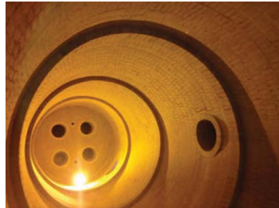
Figure 5—Sulphur furnace internals
