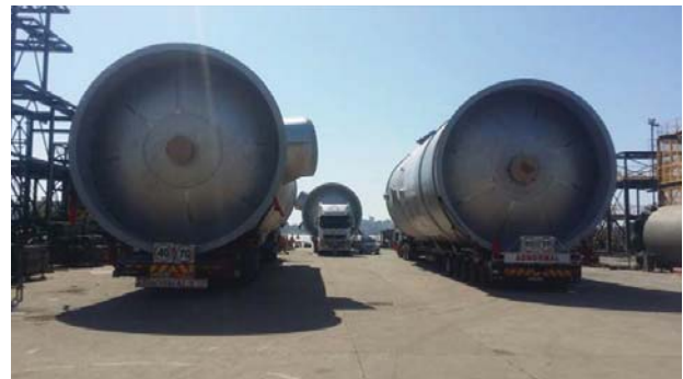
Figure 1—Completed SARAMET™ acid towers arrive at TFM site
