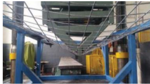
Figure 13—Test rig used to load weld mesh
