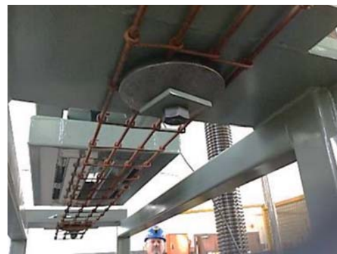
Figure 19a—Loading of a normal Osro strap
