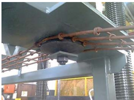
Figure 4—Dome washer clamping only some of the Osro strap strands
