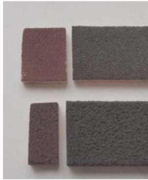
Figure 9—Colour changes of tourmaline coatings – annealed coatings are on the left. Top: FD100/SD250; bottom: FD40/SD350
