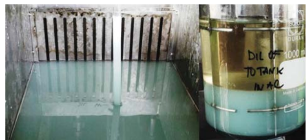
Figure 9—Aqueous continuous operation, illustrating the stable emulsion
