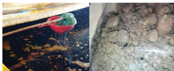
Figure 11—Crud removal in the old solvent extraction circuit, and crud from the diluent wash
