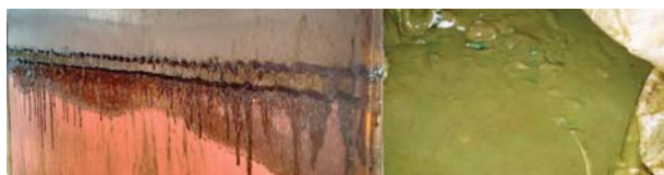
Figure 12—Crud dehydration products: organic staining (left) and siliceous 'mud' (right)
