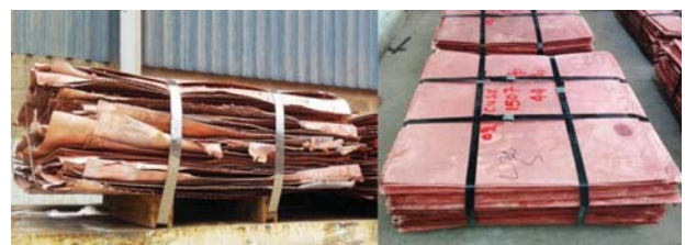
Figure 15—Physical appearance of the Luita copper cathode: before (left) and after (right) diluent wash commissioning
