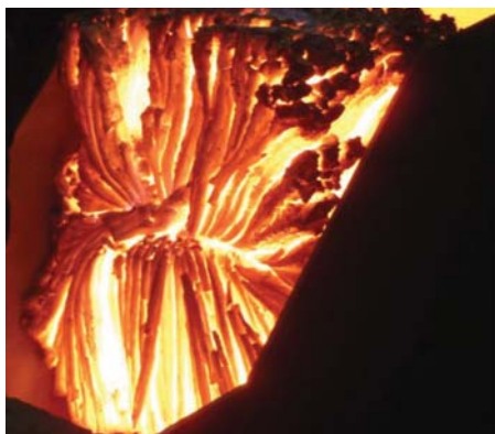
Figure 3—Successful pushing of coke into the quenching chute
