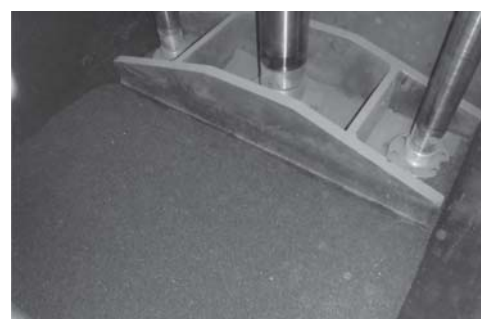
Figure 5—Hydraulic press in action inside compaction box
