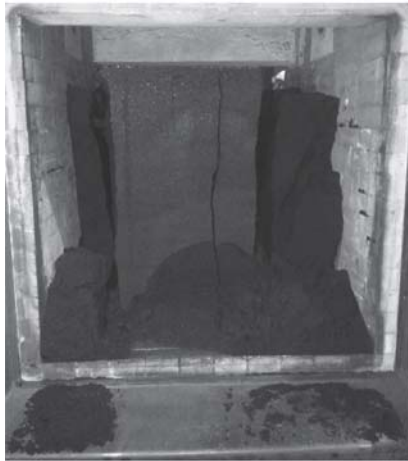
Figure 9—Collapsing of coal cake inside the pilot plant oven
