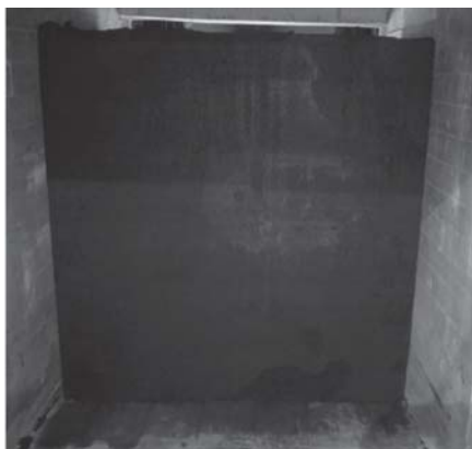
Figure 11—High-stability Waterberg ssc coal cake
