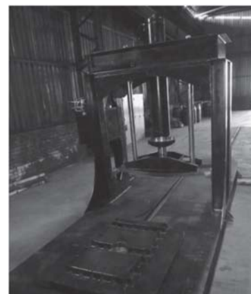
Figure 4—60 t hydraulic press with platform
