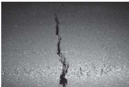
Figure 10—Large crack on top of the coal cake
