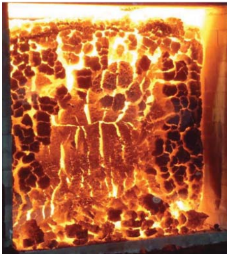
Figure 2—High-stability coke cake inside the coke oven
