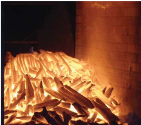
Figure 1—Coke collapsed inside the oven owing to the loading of an unstable coal cake
