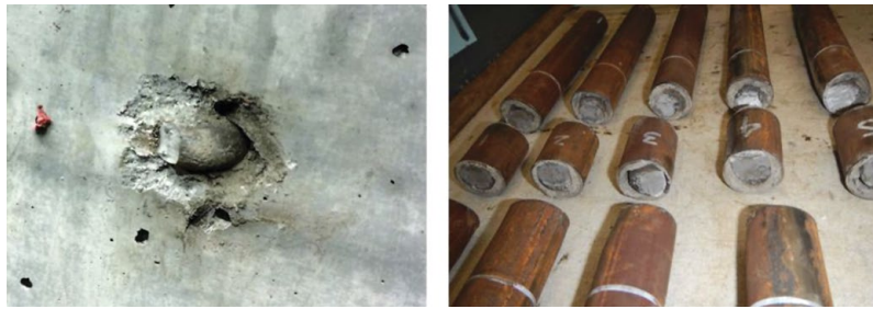
Figure 12—Post-test view of grouted PAR1 20 mm rockbolt, SINTEF/NTNU shear test on the left (SINTEF, 2017a) and the standard double shear test on the right (CSIR, 2016a)
