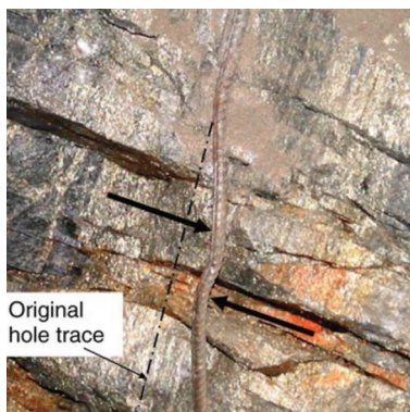
Figure 16—A rebar bolt exposed on the advance face of a cut-and-fill mine stope. The bolt was subjected to shear loads and deviated from its original hole trace. The thick arrows point the direction of possible shear movements in the rock (Li, 2009)
