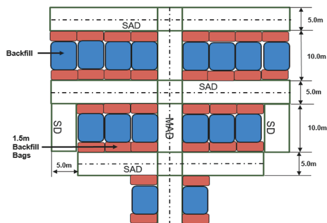
Figure 6—Plan view of the horizontal destress layout
