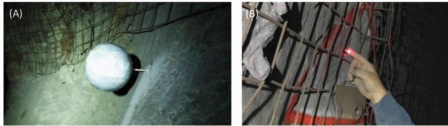
Figure 3—(A) A survey sphere is placed on the wall. (B) Either the collar or the sphere centroid location is known, so the point cloud can be referenced to these locations
