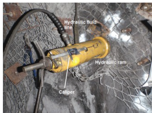
Figure 2 – Example of a typical in-situ pull test set-up. Note that the rebar protruding from the hydraulic ram is not the rockbolt being tested, but is rather a pull rod connected via an adapter or claw type attachment
