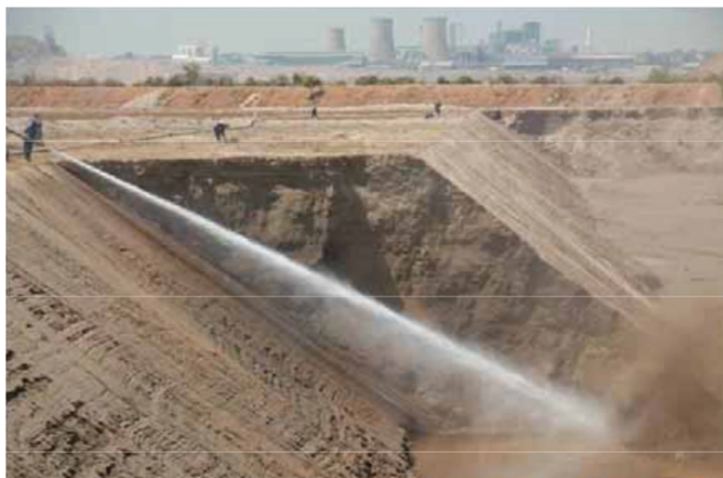
Figure 6—Mining at a 45° angle (Garling and Prentice, 2010)
