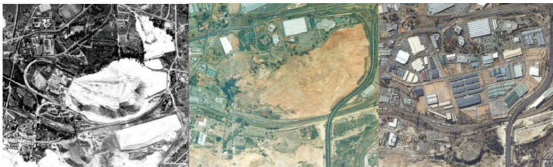
Figure 7—Sequence of rehabilitation through mining (left to right, tailings dam, re-mining site, industrial site) (DRDGold IAR, 2017)
