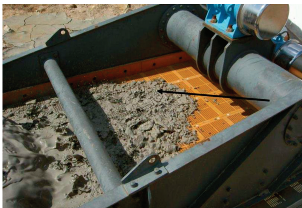
Figure 5—Example of vibrating screen to remove debris from the slurry (Fraser Alexander, 2012)
