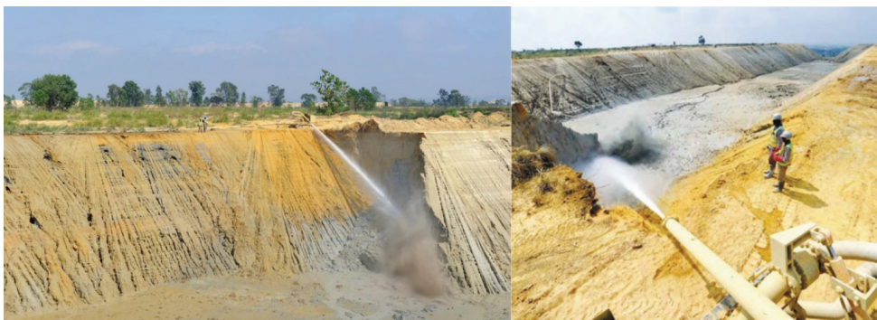
Figure 3—Examples of hydraulic mining of a TSF/tailings dam (DRDGold IAR, 2017)
