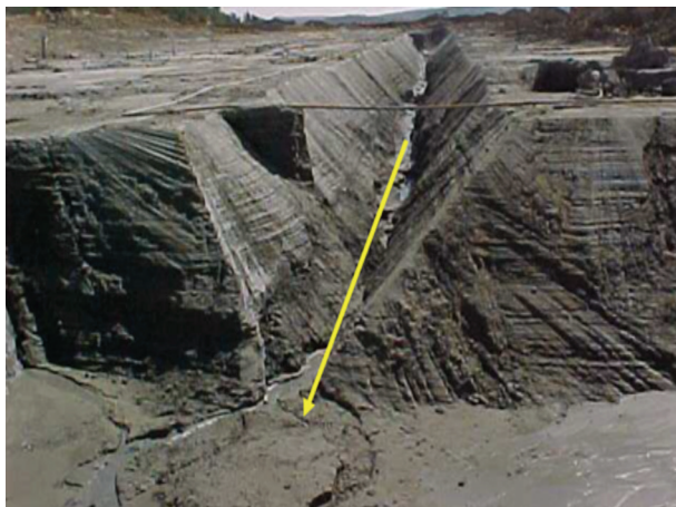
Figure 4—Gully used to transport slurry (Fraser Alexander, 2012)
