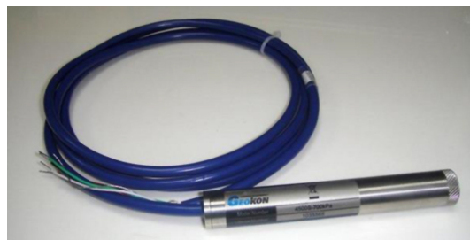
Figure 2—Example of a vibrating wire piezometer prior to insertion (Morton, 2020)
