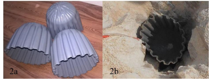
Figure 2—Stemming plug 1. (a) Plastic mould, (b) installation in blast-hole
