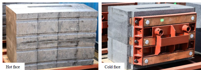
Figure 2—Copper-graphite composite cooler assembly (Joubert et al., 2024a)
