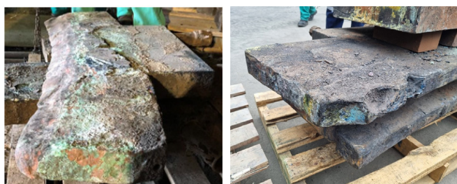
Figure 1—Examples of localised attack on exposed copper surfaces
