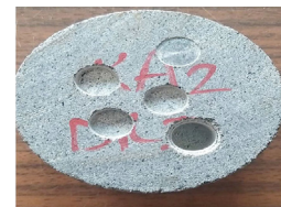
Figure 6—A rock sample after the SJ test
