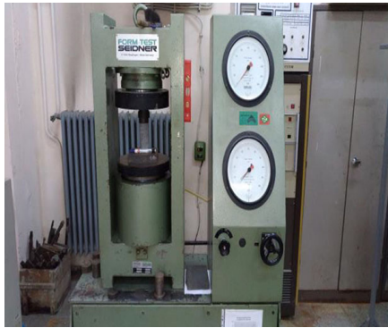
Figure 2—Hydraulic press used for the strength tests
