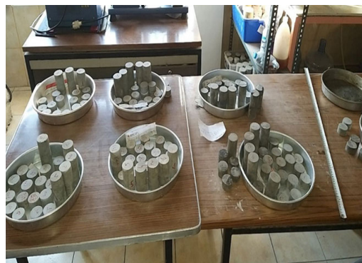
Figure 1—Core samples prepared in accordance with standards
