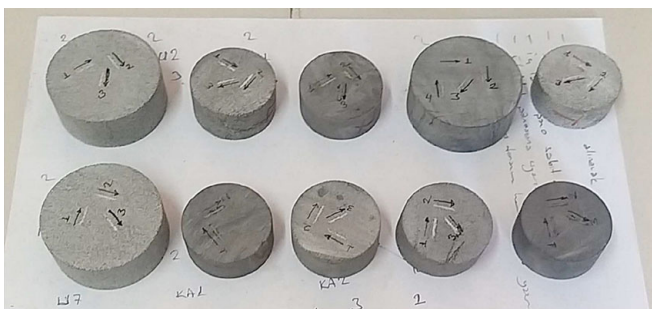
Figure 11—Some rock samples subjected to the CAI test
