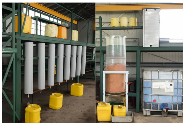
Figure 6—Laboratory and pilot-scale column leaching setup used for cobalt recovery trials. Left: array of 5 L acrylic columns mounted on a modular frame for parallel batch testing. Right: 200 L transparent PVC column packed with oxidised ore for pilot-scale validation. Yellow containers collect pregnant leach solution (PLS); intermediate bulk container (IBC) stores recycled leachate. Setup supports RTD testing, reagent recirculation, and scale-up of AR-derived reactor configurations
