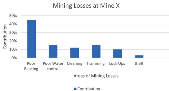
Figure 2: Root causes of poor Mine Call Factor at Mine X. Derived from survey and interview data showing key contributing factors such as blasting inefficiencies, water control issues, and cleaning delays
