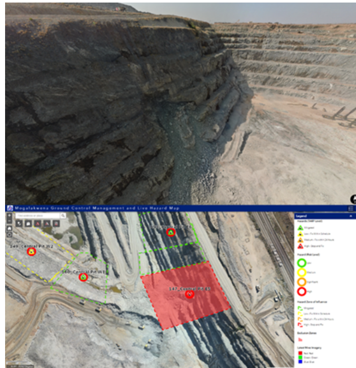
Figure 10. Example of live hazard map showing risk level and TARP level and zones of influence / no-go zones.
