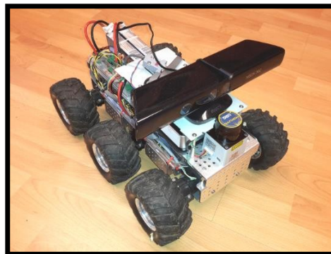
Figure 4. The WMR (Tóth et al. , 2015). A remotely operated vehicle (a land-based option) for consideration in the pursuit of optimising incident investigations in the context of South Africa
