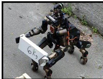
Figure 7. An example of a hybrid robot – a wheel-legged robot (Kashiri et al., 2019)
